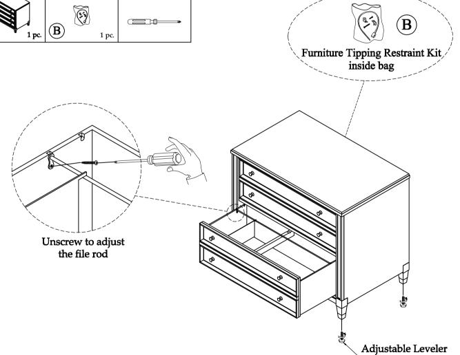
For product and personal safety, a Anti-Tip Restraint Kit has been included with this cabinet which can help to minimize the risk of the cabinet accidentally tipping forward, if used and properly installed
